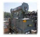
GridON's FCLs are being installed both in transformer feeder locations and in bus-sections. They can also be installed on generator feeders, since they can be rated to the full capacity of the generation source and never interrupt the current during fault. The FCL instantly suppresses excessive current and recovers to normal load immediately upon fault clearance - being always ready for consecutive short circuit
